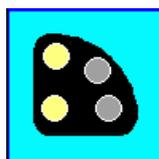
On seeing a “proceed with caution” on signal 32, drivers should attend to the dwarf signals, even when they are passing through a station (i.e. not carrying out shunting movements).
